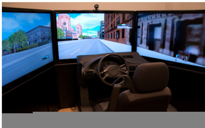
Fig. 1. The VS500M car driving simulator (Virage Simulation Inc. ® ) used in the present study.
